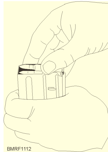
Figure 11-12.—Loading cartridges into the magazine, 20 -round capacity.
